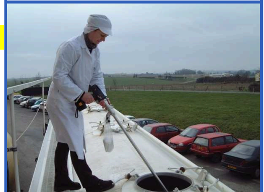
Vertical sampling in a sachet from bulk tanks with a 1500mm Long sampler Ref. S7PV15R
